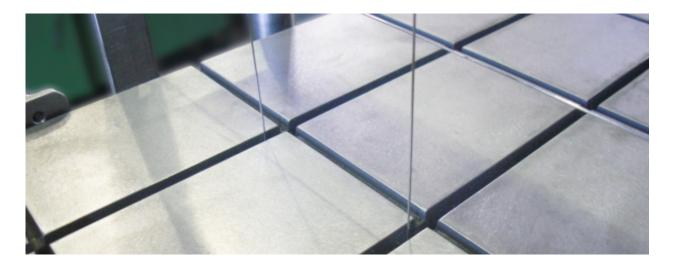
The equipment provides an even cut of a layer of cheese, butter and other plastic products using an adjustable stop.
