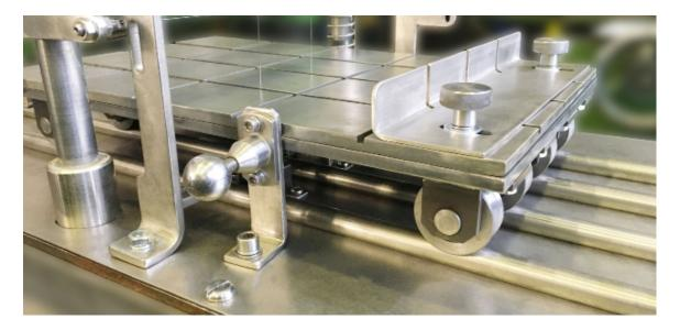
Cutting the product using the «String» device with adjustable tension. A slot on the table for easy cutting into the same shape.
